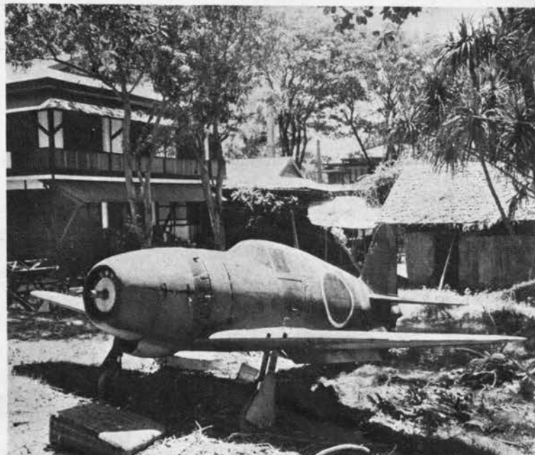
JACK Overall roundness marks barrel-shaped navy fighter. Tail is rounded and tailplane is set well forward of rudder. A later model has bubble canopy in place of faired cockpit shown here.
